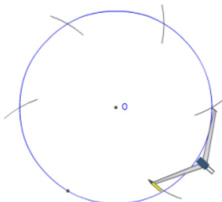
6. Draw a line between each successive pairs of vertices, for a total of six lines.
