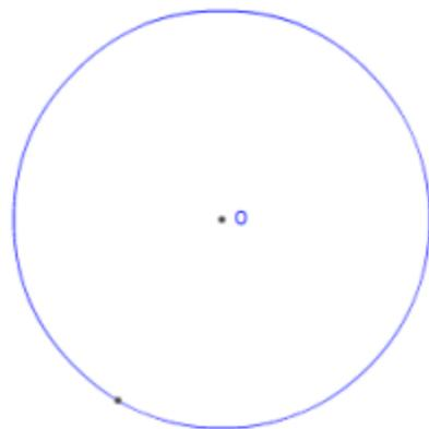
2. Set the compass on point P and set the width of the compass to the center of the circle O. The compass is now set to the radius of the circle  $\overline{OP}$ .
