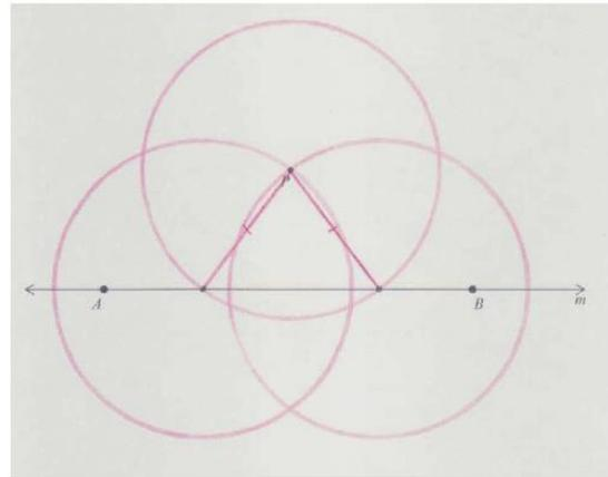
*Construct the perpendicular bisector of this line segment by drawing two congruent circles with radii that are more than half the length of this segment using the intersections shown in the previous step as the centers.*
