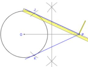
6. Done. The two lines just drawn are tangential to the given circle and pass through P.
