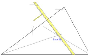
8. Place the compass on the incenter and set the width to point M. This is the radius of the incircle, sometimes called the inradius of the triangle.
