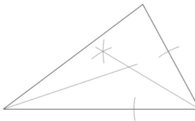
6. Where the two new lines intersect, mark a point as the incenter of the triangle.
