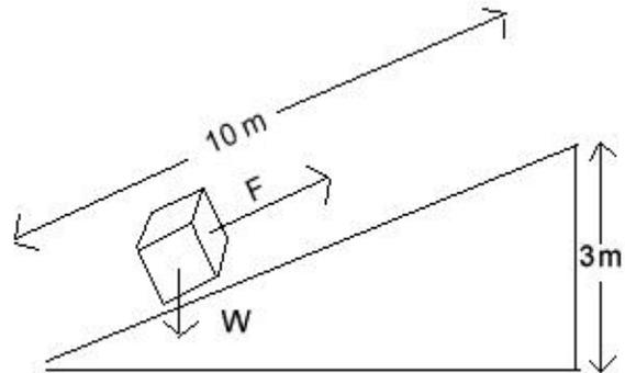
Determine the mechanical advantage of the ramp.
