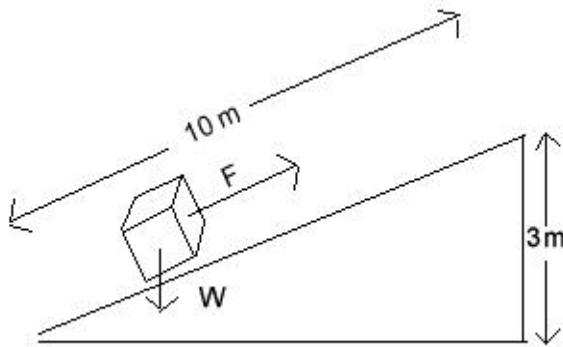
Determine the mechanical advantage of the ramp.
