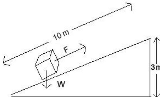
Determine the mechanical advantage of the ramp.
