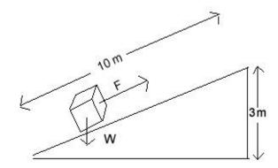
Determine the mechanical advantage of the ramp.
