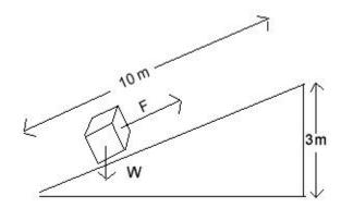
Determine the mechanical advantage of the ramp.
