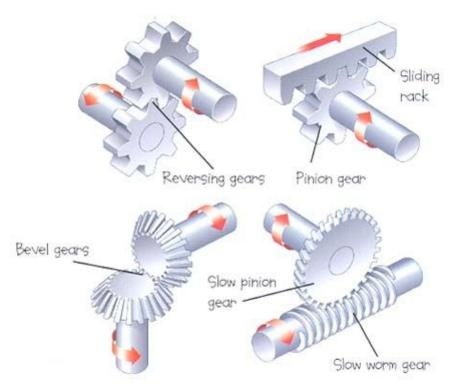
Gears change the turning direction of a force. They can slow it down or speed it up--and even convert it into a sliding force (rack and pinion).
