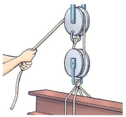
Two pulleys together reduce the force needed to lift a heavy girder by one half.
