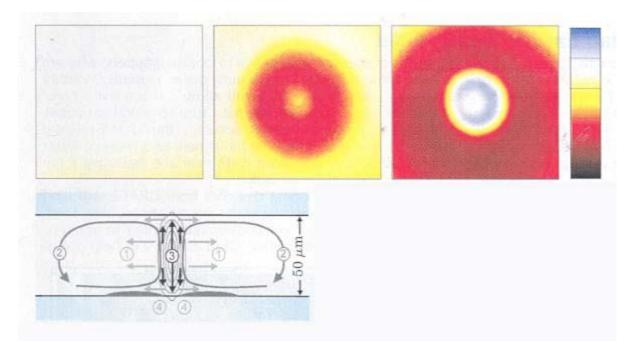
DNA is trapped when the container is thick enough for convection to occur. The three top images, which are taken from above the container, show how the intensity of fluorescent dye changes after the onset of heating. In the linear color bar, black represents zero intensity; blue represents the maximum. The sequence runs from left to right and corresponds to intervals of 0 s, 10 s, and 60 s. In the last image, the blue ring-like
