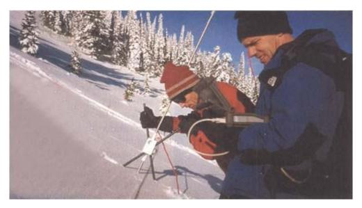
A probe called the SnowMicroPen helps avalanche scientists detect leak layers of snow near the bottom of a snowpack.
