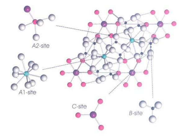
Figure 2. Ball-stick representations of the apatite structure: (001) projection, and the A, B, and C atomic sites. There are two distinct A-sites, labeled A1 and A2, which are normally occupied by Ca. The complete coordination spheres of the A2 and B sites are not visible in this orientation.
