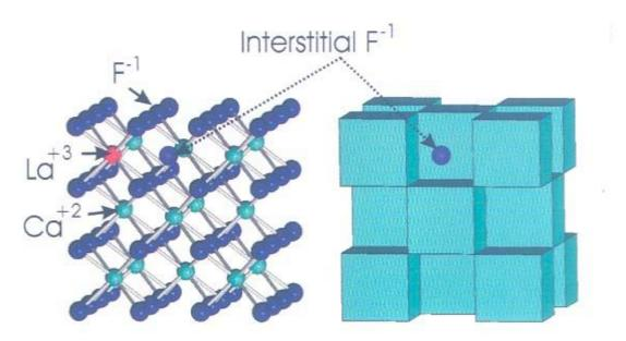
Figure 3. Ball-stick (left) and polyhedral (right) representations of the fluorite structure. The
